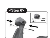
6.Loosen the bolt and nut by a first. Then place the handle bar over the front wheel stick,insert the bolt into the hole and tighten by the nut.
