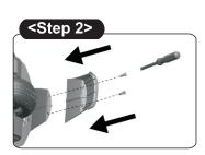
2.Place the rear fender over the location in the rear body, tighten by two screws with a screwdriver(not included).
